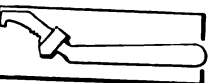
Fig. 4—Type of adjustable spanner which will be found to be a handy tool about the car
